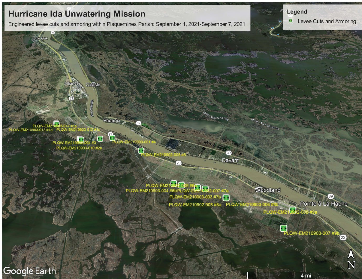
Figure 2: Engineered levee cuts and armoring within Plaquemines Parish, LA
